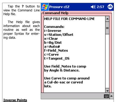
Tap the Command Line text box to begin. The popup keyboard will appear. Tap the I key and the word **Inverse** appears in the text box with a space after it. Now just enter the two points you need to inverse, separated with a space.
