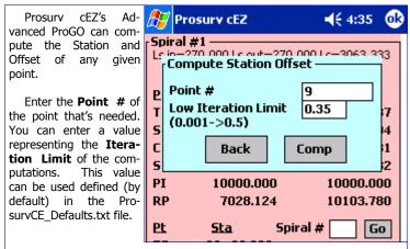
In order to find the station/offset, the point must lie somewhere within or offset from the Geometry of the Spiral-Curve-Spiral.
